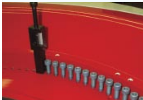
Each MGC air ring comes with a gauge that helps determine your adjustments
