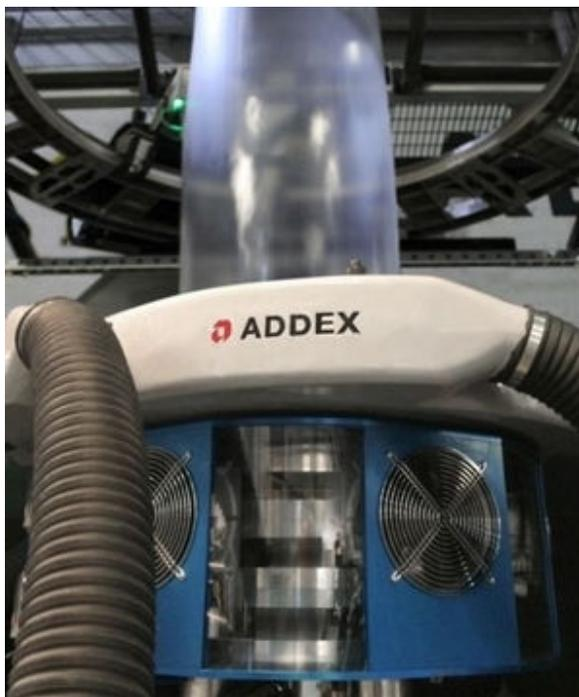
**Düsseldorf, Germany** — Newark, N.Y.-based maker of cooling technologies for blown film extrusion Addex Inc. exhibited two new products at K 2016. Both were air rings featuring the company's Intensive Cooling Experience (ICE) technology.
